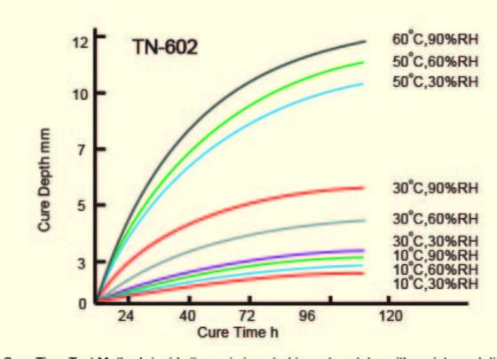
Cure Time Test Method:riquid silcone is inserted in a glass tube with an intermal diamater of 10mm, and measurements of the cure length are taken at specifie intervals.
